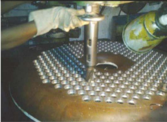
KNUCKLE TUBESHEET (J) PREPARATION ON RADIAL DRILLING MACHINE
