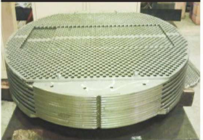
BAFFLE STACK IN READY TO USE CONDITIONS
