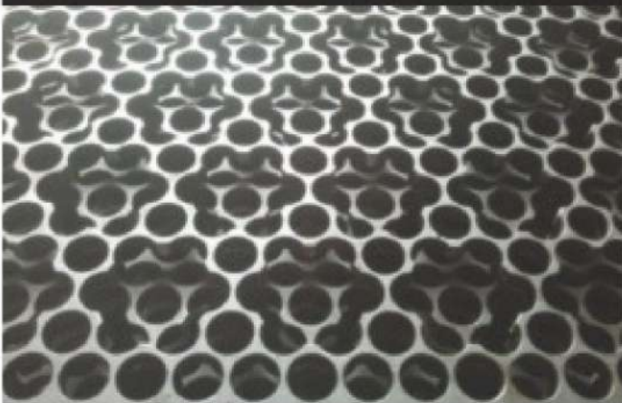
REACTOR BAFFLE WITH ORIFICE HOLES CUTTING
