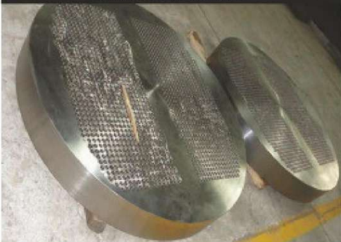
TUBESHEET DRILLED ON CNC BTA DEEP HOLE DRILLING MACHINE
