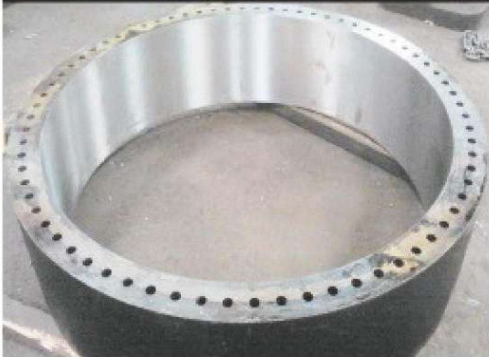
THREAD LOCK RING DRILLED ON DEEP HOLE DRILLING MACHINE
