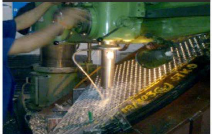
HELICAL BAFFLES DRILLING WITH FIXTURE
